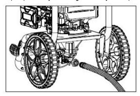
The minimum recommended length for the water supply pipe is 10 meters (but not more than 25 meters) with a diameter of 12.5 mm to avoid back pressure and any potential damage to your appliance. Make sure it can withstand water and a maximum pressure of 10bar (0.1Mpa). If you want to connect your device to other water sources, make sure the maximum water inlet pressure is 10bar (0.1Mpa).
